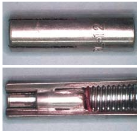
Typical Drop-In Anchor (Full Sectional) Failure of ½-inch drop-in anchors were the topic of the University of Toledo Engineering Department Student Project.
