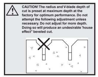
The blade is preset to the proper cutting depth at delivery. Little or no adjustment is necessary.
