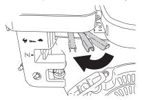
· Close the engine choke lever.
