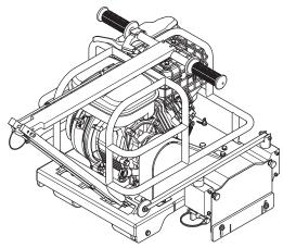
Raise the blade by pushing down on the handle bar with both hands to the full and locked position. Remove the blade block guard.
