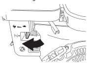
The closed choke position enriches the fuel mixture for starting a cold engine.
