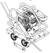
Insert one the two wrenches supplied, in the slot at the front of the engine and one on the blade shaft bolt.
