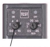
To adjust the amount of time that the Auto Drain Valve is open.
