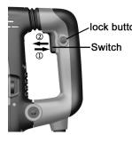
• The trigger-style switch starts the hammer; lock button depressing the lock button will lock the trigger •Switch in the ON position.
