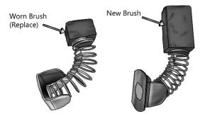
To re-install the brushes or replace with a new set, the brush should be inserted into the brush carrier subassembly, the lead wire connected, and the spring clip (coil spring) should be repositioned to firmly hold the brush into place. The wire lead must be reconnected to the wire lead connector.
