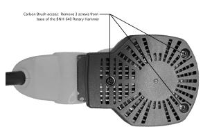
Carbon Brushes are subject to wear over time. Brushes should be inspected after every 100 hours of use. At least 1/4" of the wearable surface should remain for the tool to perform optimally.
