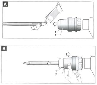
Slide the front of the chuck toward the body of the tool to insert, lock, and release an SDS Max bit
